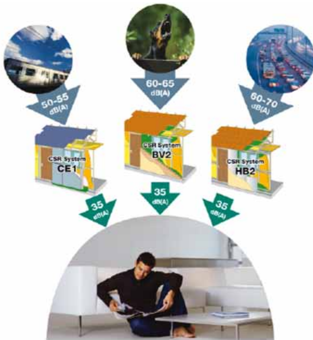
Fig. 9.1 Interior Noise Level Reduction Through CSR Sound Control System
